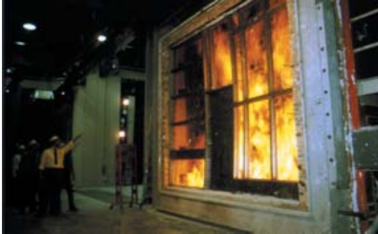
Photo 3. UL fire science engineers evaluate a glass wall.
