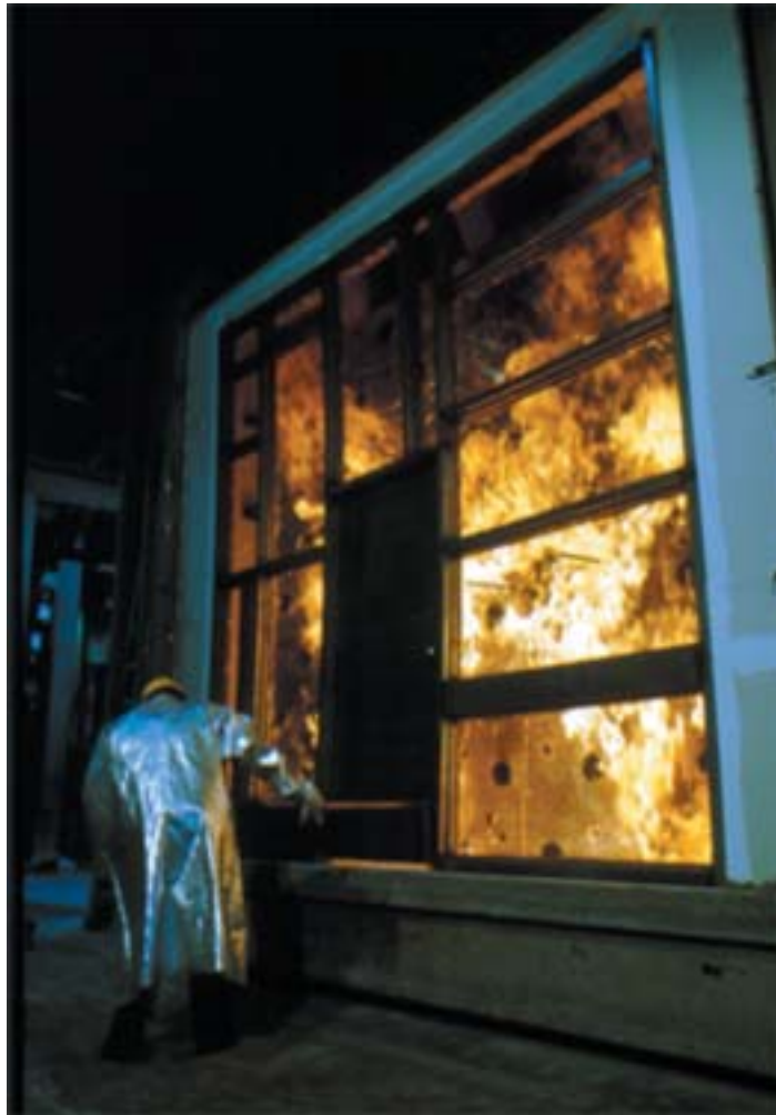
Photo 2. A glass wall assembly being subjected to 2000 degrees of heat.
